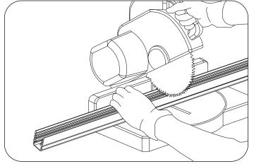
**2** Take reduced measurements and cut cap rail housing to length with chop saw. If using frosted lens, cut lens to same length as cap rail housing. Do not cut both at same time.
