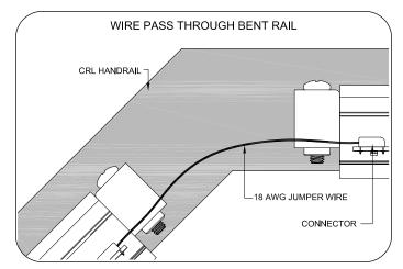
**11** Use 18 AWG jumper wire to accommodate angled rails. The connectors are designed for use with stranded and solid core 18 AWG. Inserting stranded 18 AWG wire into connectors is easier if wire is lightly tinned.
