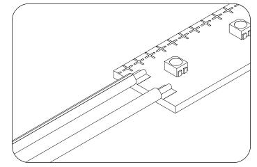
6 If the cut piece is in middle of run, prepare LED strip light by using a soldering iron tip with solder to burn off transparent waterproof coating at LED strip light cut lines. Then solder 18 AWG jumper wires to cut LED strip light to connect to adjacent LED strip light. Note: The black & white striped wire is positive (+) and black wire is negative (-).
