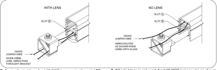
7 If using frosted lens, feed 18 AWG jumper wire through LED mounting clip as shown (above left), and slide clip in cap rail into Slot (B).
