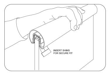
13 If using handrail with glass, insert handrail with completed cap rail housing and LED strip lights onto glass once all the above steps are completed. Glass enters base of cap rail housing and stops at interior housing tabs. Note: If loose after glass insertion, cut LED housing shims to size and insert between glass and housing.
