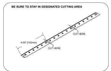
5 The LED strip light is designed to be cut in 4" (102mm) lengths as indicated by the double lines on the LED strip lights. Use a hack saw or other fine toothed saw to cut the LED strip light. If cut LED strip light is used at the end of run, no soldering is required. Note: the remainder LED strip light is usable elsewhere if needed.
