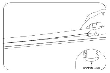
**12** Gently snap on frosted lens at end of cap rail housing. Continue to press frosted lens down length of housing channel, snapping it securely in place.
