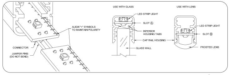
3 Slide LED strip lights into cap rail housing slot. If using with glass, place LED strip light into slot (A). Slot options (A) or (B) are available if using with frosted lens. Once inserted, take two jumper pins and insert into female connectors on end of LED strip light. To connect LED strip lights, align the "+++" of the first board to the "+++" on the second LED strip light board.
