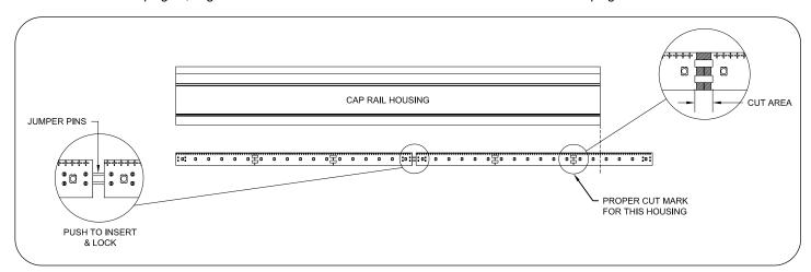
4 Slide LED strip light into the extended jumper pins until strip lights link securely together. Custom cut option is described in Step 5.
