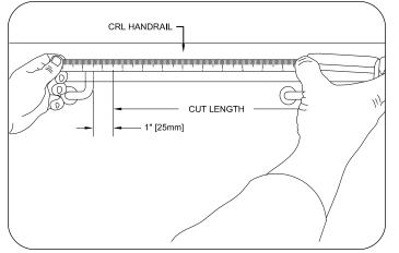
1 Measure the distance between handrail supports. Subtract 2" (51mm) total from the measurement to allow for clip space.
